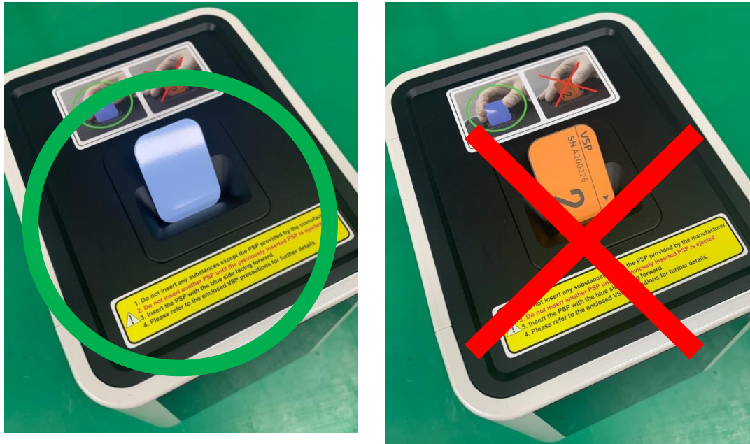
Figure 12. How to insert the Phosphor Storage Plate
